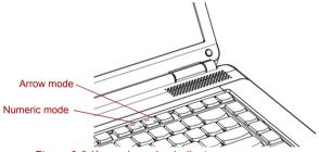
Figure 2-9 Keypad overlay indicators
